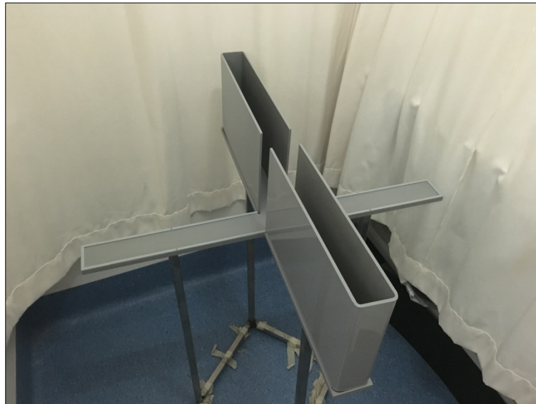
Figure 3: Elevated Plus Maze Apparatus. The apparatus used in the current study was a '+'-shaped maze which consisted of two enclosed arms and two open arms; all arms extending from a central platform. The maze was raised at a height of 70 cm from the ground. Each animal was placed on the central platform facing one enclosed arm and allowed to explore the maze for 5 min.
