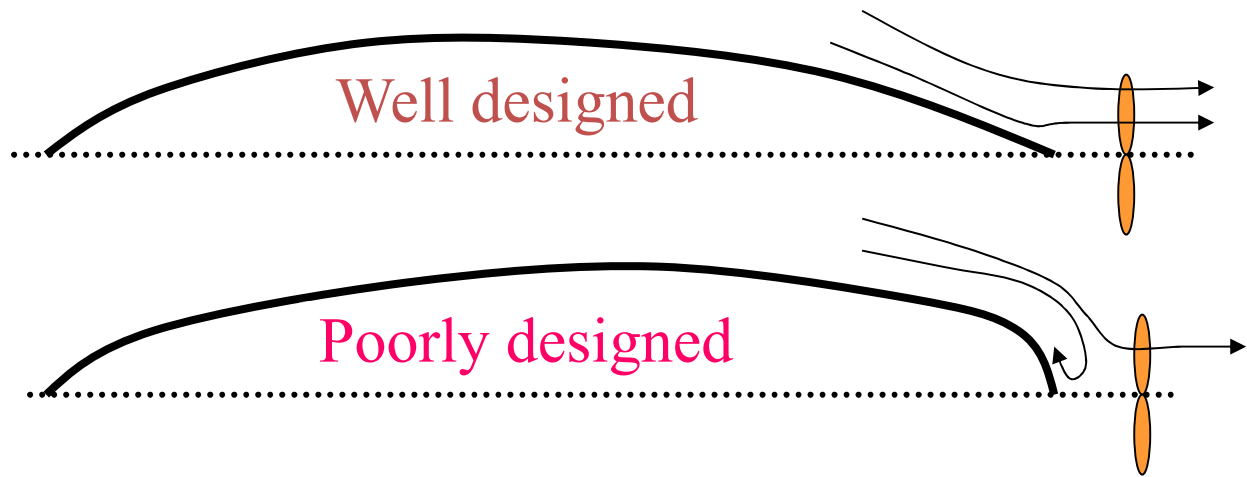
Figure 7: Flow behavior at aft of UUV
