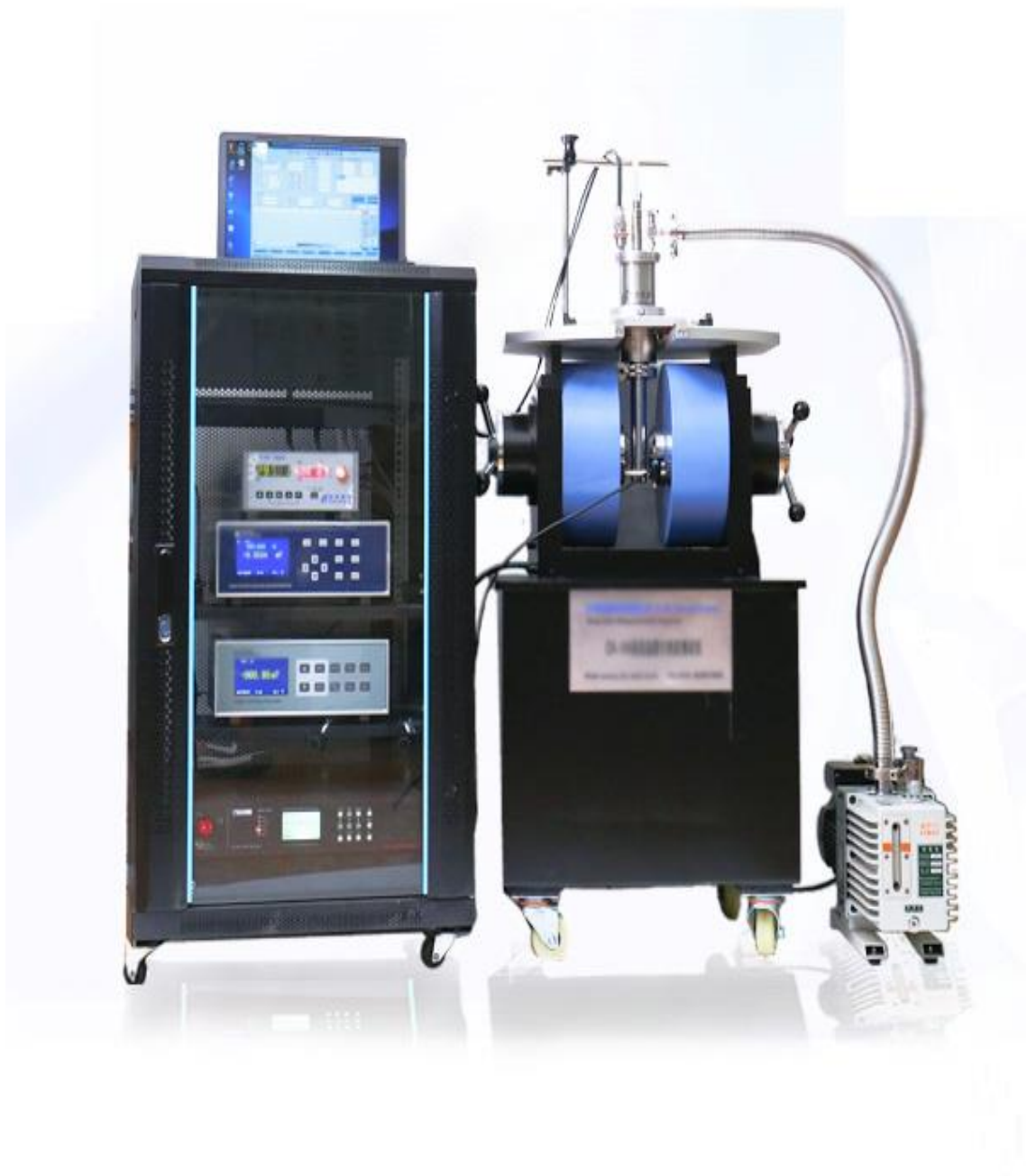
Figure 3.11 Hall Effect Measurement System [96]
