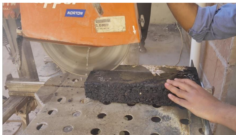
Figure 3- 22 Slab cutting by diamond saw for beam preparation
