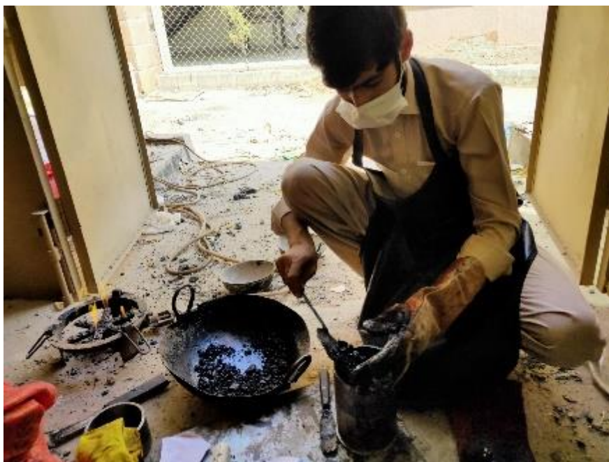
Figure 3- 29 IDT sample mixing and pouring in mould for compaction
