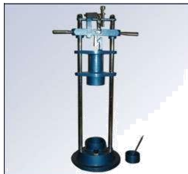
Figure 3- 11 Aggregate Impact Value Test
