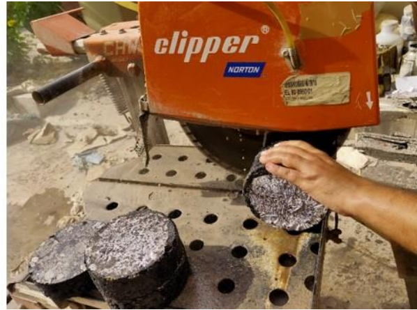
Figure 3- 31 Prepared Gyratory samples (all combinations) and their cutting by diamond cutter
