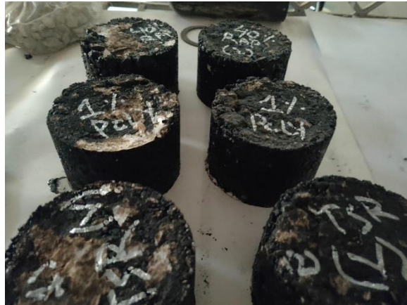
Figure 3- 32 All (conditioned & unconditioned) samples of IDT test
