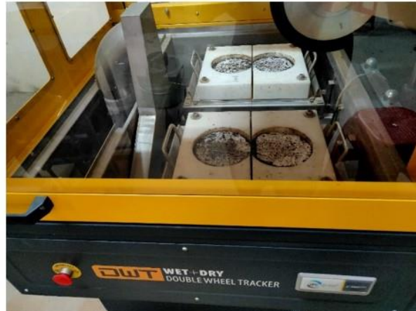
Figure 3- 28 Sample placed in DWT (double wheel tracker) for Rut test
