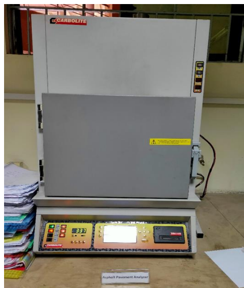
Figure 3- 7 RAP binder content findings by ignition method
