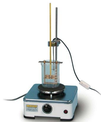
Figure 3- 15 Softening Point Apparatus
