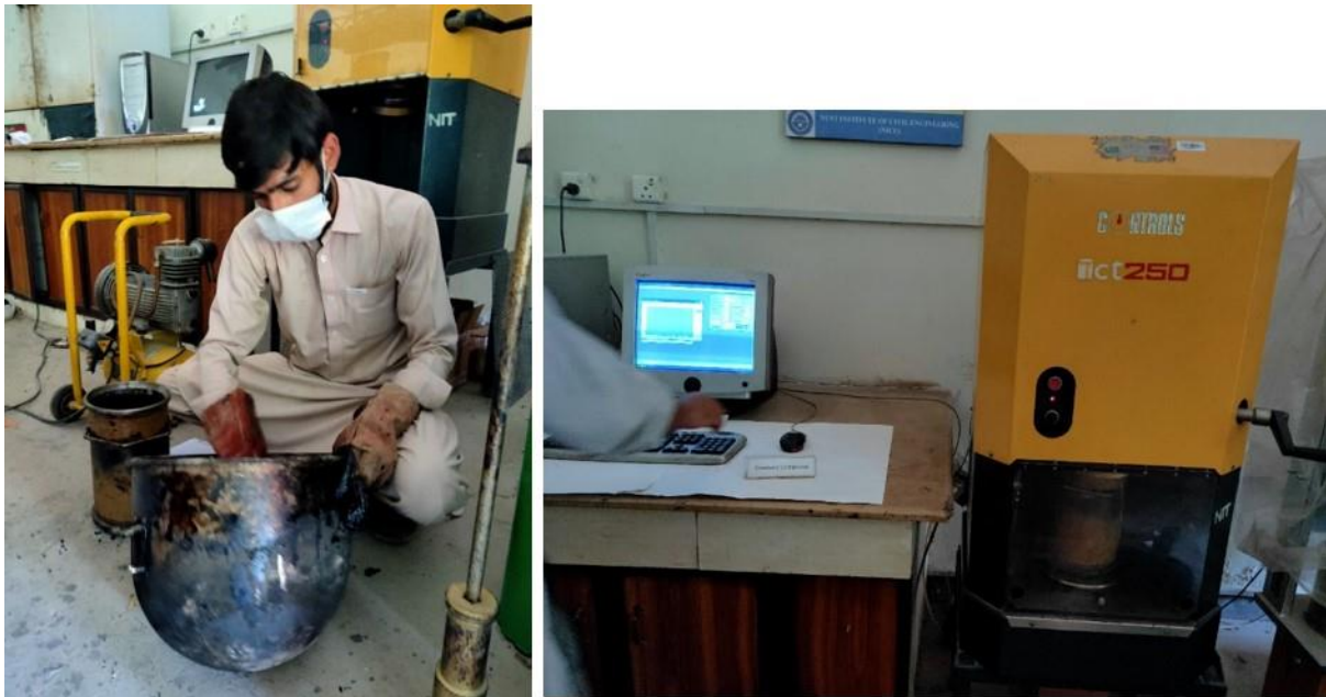
Figure 3- 27 Preparation and Compaction of Gyratory Molds for DWT
