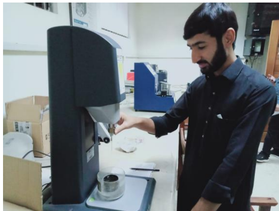
Figure 3- 14 Penetration Test being performed on Penetrometer Apparatus
