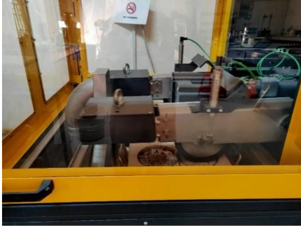
Figure 3- 28 Sample placed in DWT (double wheel tracker) for Rut test
