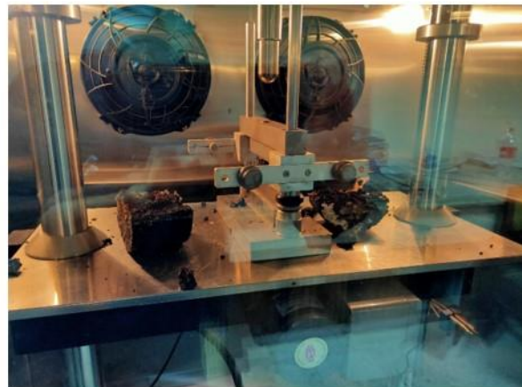
Figure 3- 30 a) Sample placed in UTM for IDT test, b) Sample after performing IDT test
