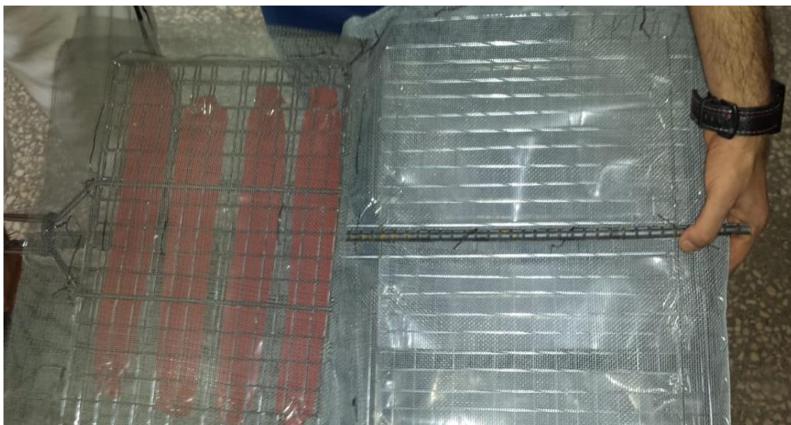
Figure 2: A) High Density Polyethylene (HDPE) Strip, B) Cage of HDPE used for the deployment of passive sampler, C) Deployment of Polyethylene(PE) passive sampler at a water site by IESE,NUST team using BBQ grill as a cage.
