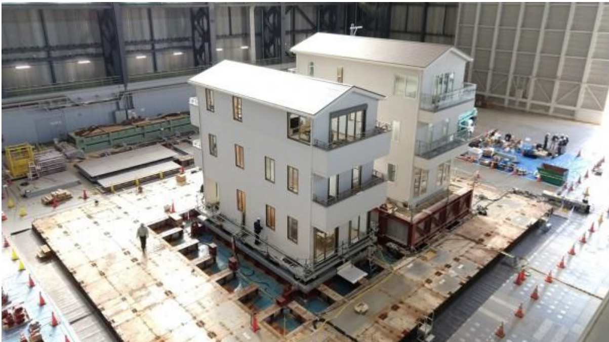
Figure 5 Shaking table assembly for testing
