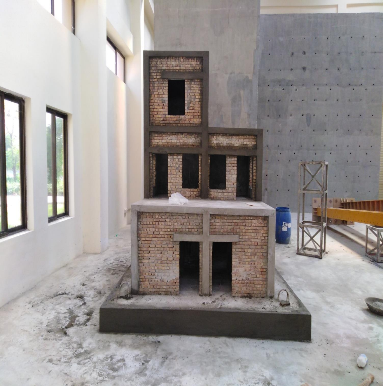
Figure 33 Confined Masonry Structure
