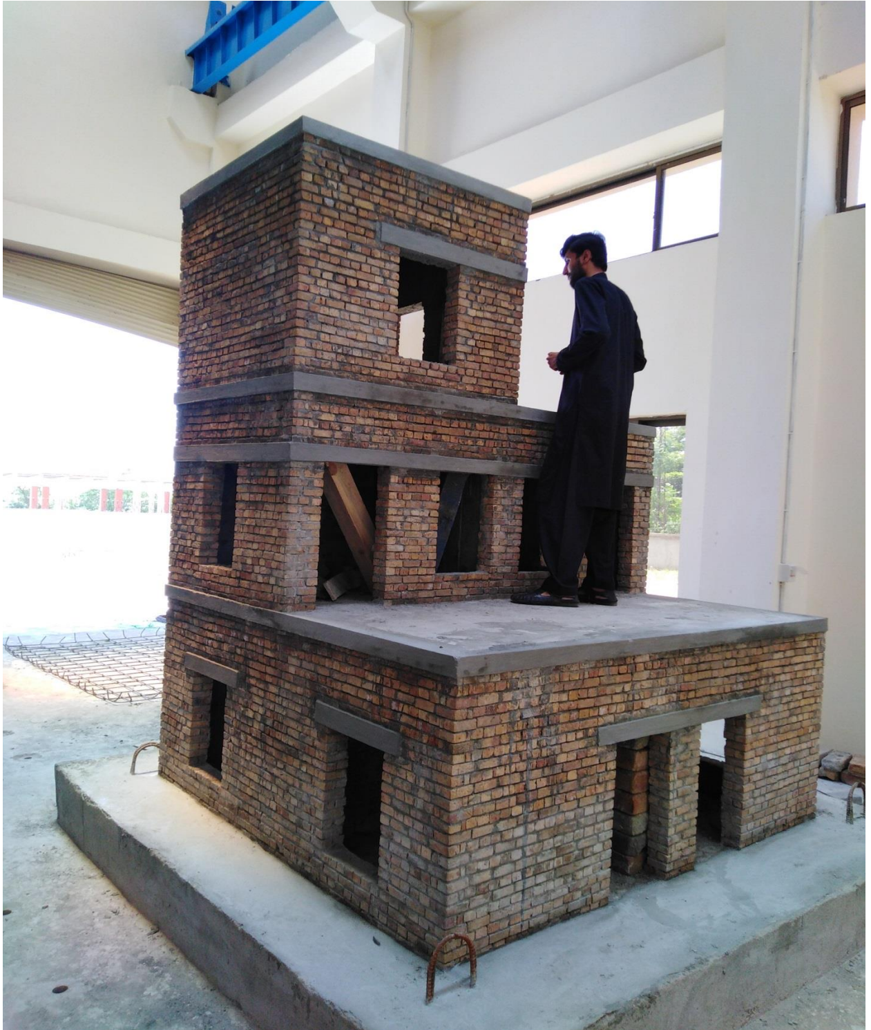
Figure 31 Unconfined Masonry Structure Model
