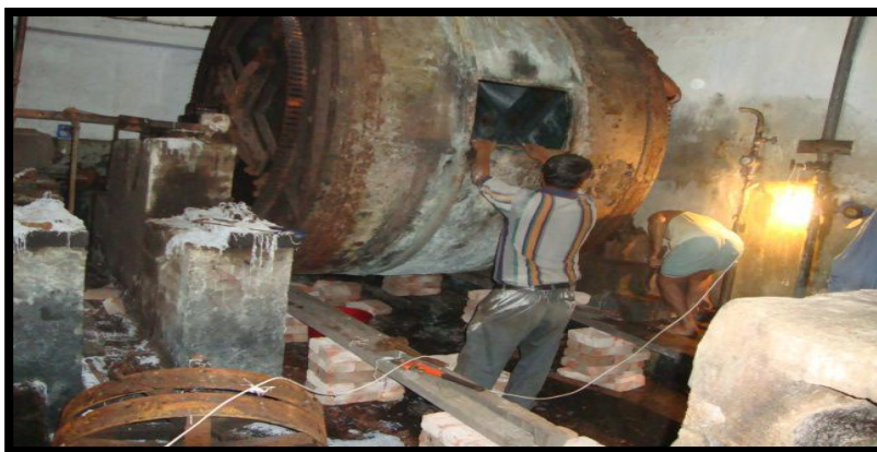
Figure 2.4: Liming process done in a drum for unhairing
