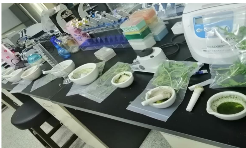
Figure 3.10: Grinding leaves for sample preparation for spectrophotometry
