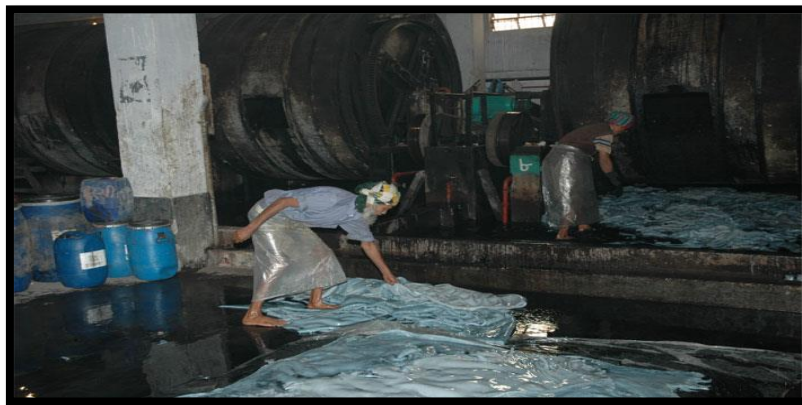
Figure 2.3: Soaking of raw hides in alkali solution for unhairing
