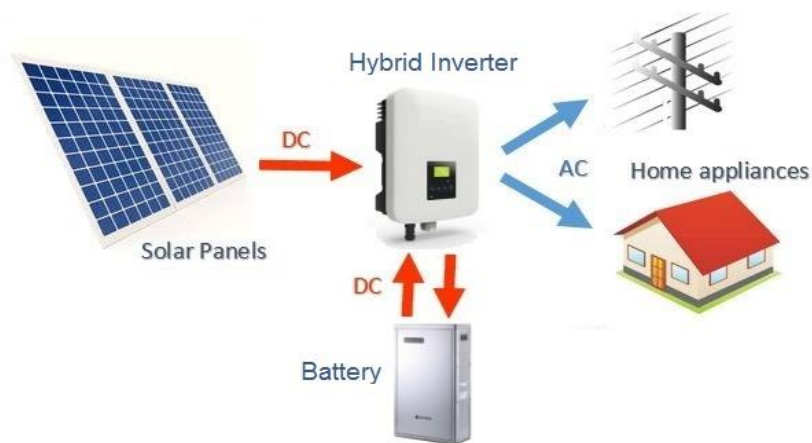
Figure 2-11: Basic layout of a hybrid PV system [52]
