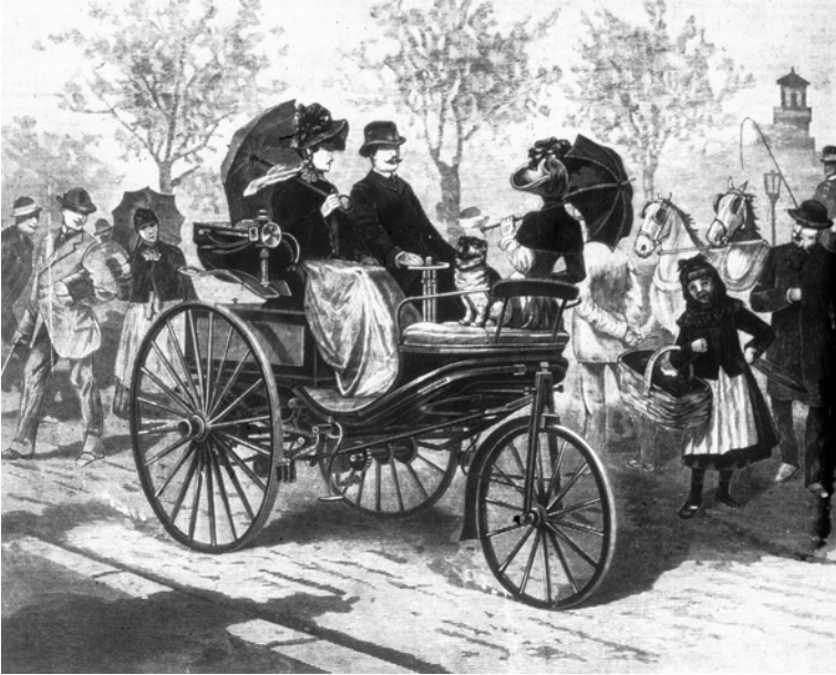
Figure 2.10 Gasoline-powered three-wheeler by Benz & Cie., as shown at Munich machinery exhibition in 1888. Reproduced from Scientific American , January 5, 1889.
