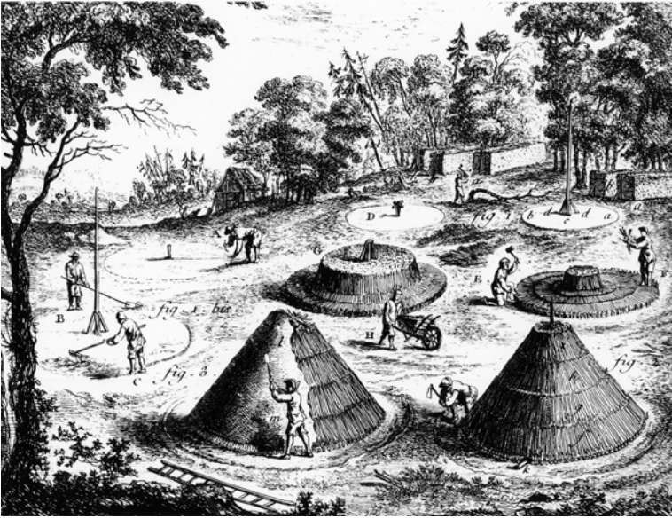
Figure 1.1 Steps in preparing wood piles for charcoaling illustrated in Diderot and D'Alembert's L'Encyclopédie (1769–1772).
