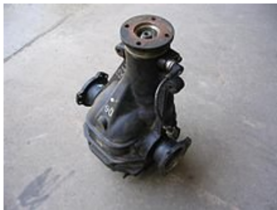
Figure 9 Nissan 240SX Viscous LSD
