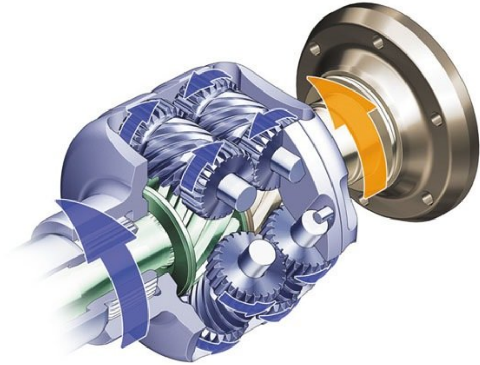
Figure 10Torsen T1 LSD
