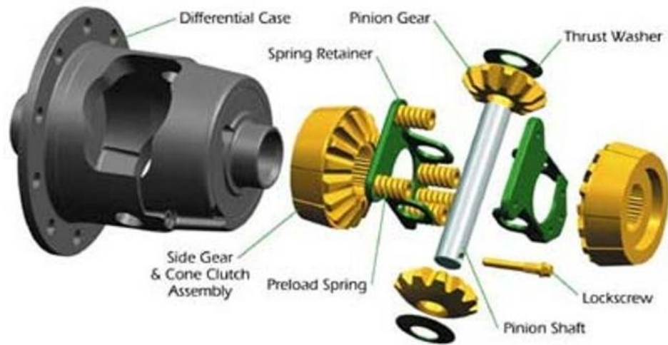
Figure 12 Cone clutch differential
