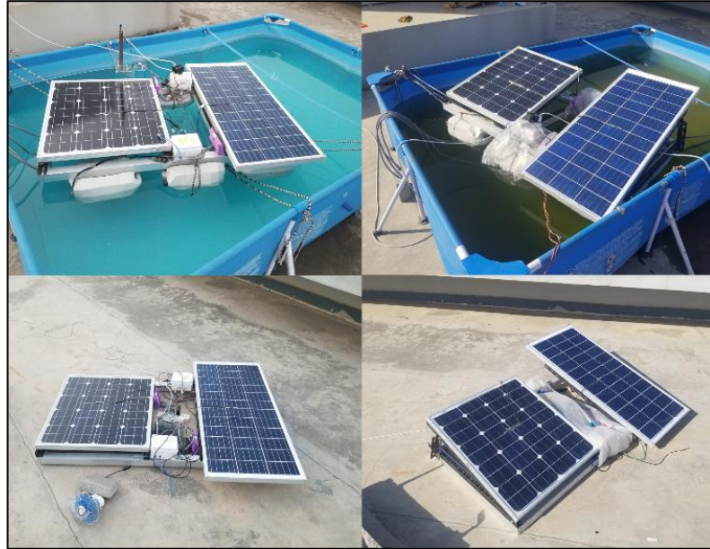
Figure 3.2: Configuration of FPV and OPV system
