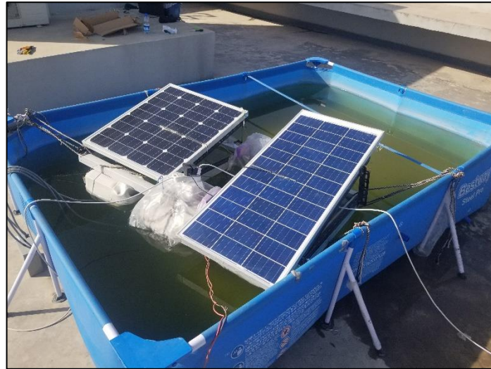
Figure 4.2: Partially Covered Evaporation Test
