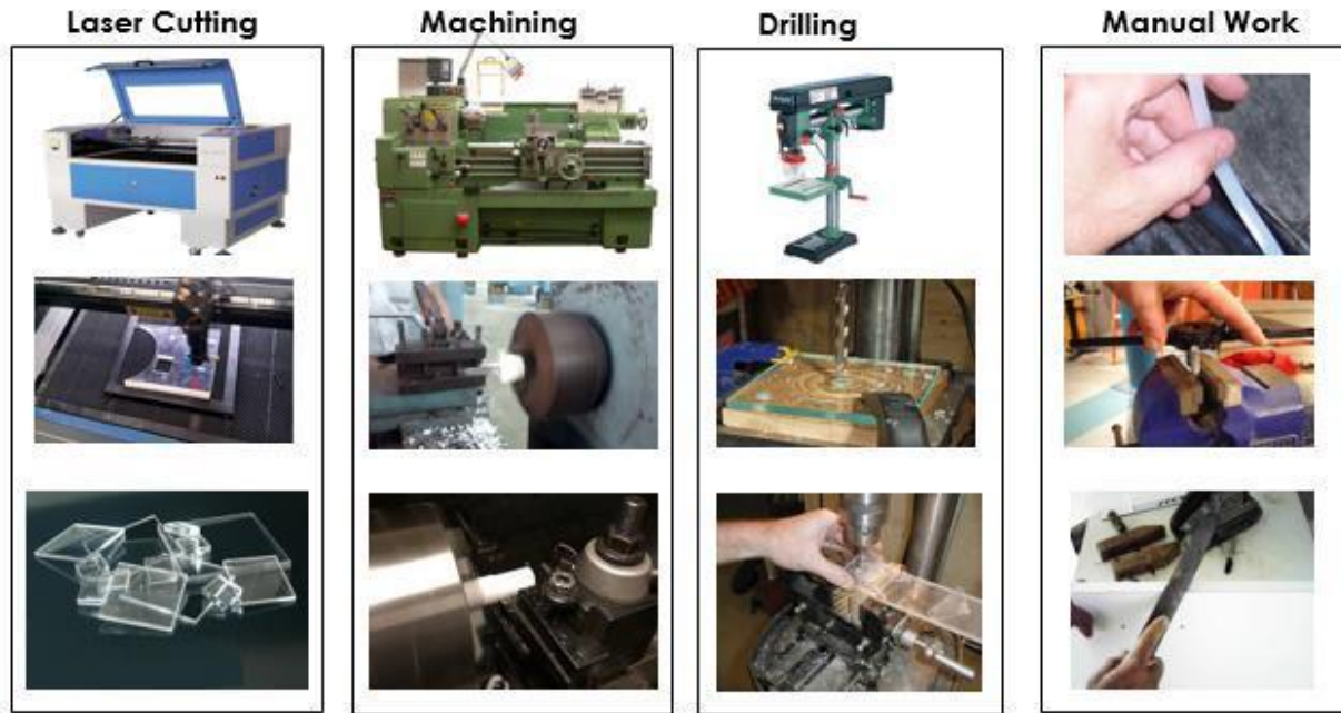
Figure 8 Techniques involved in the fabrication of subcomponents of the Stent Migration Testing Rig
