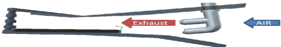
Figure 2.2 Air flow through Ejector
