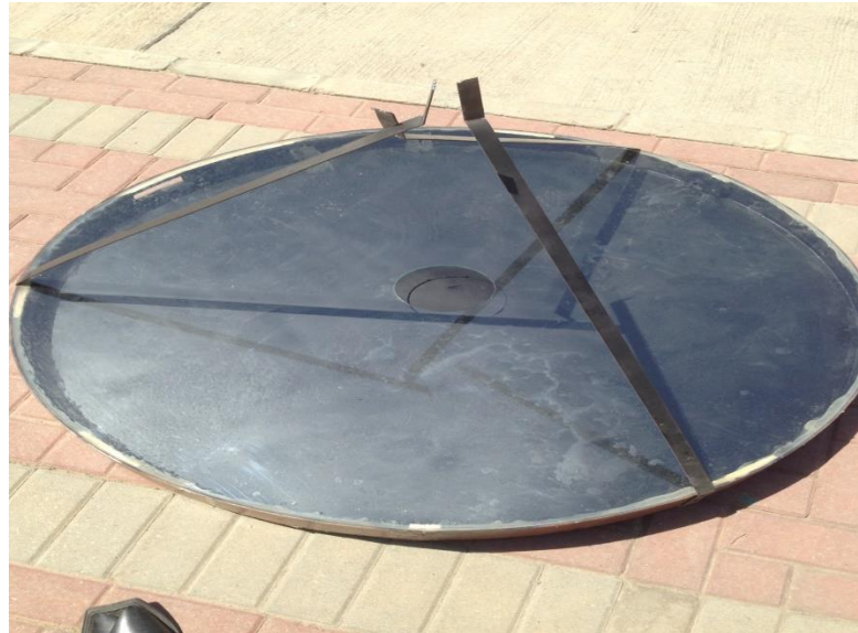
Figure 2-4: Solar Air collector (One we fabricated)
