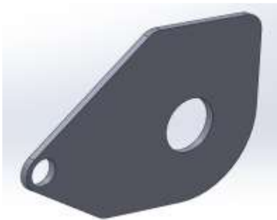
Fig 7.2: Generator Mounting Plate
