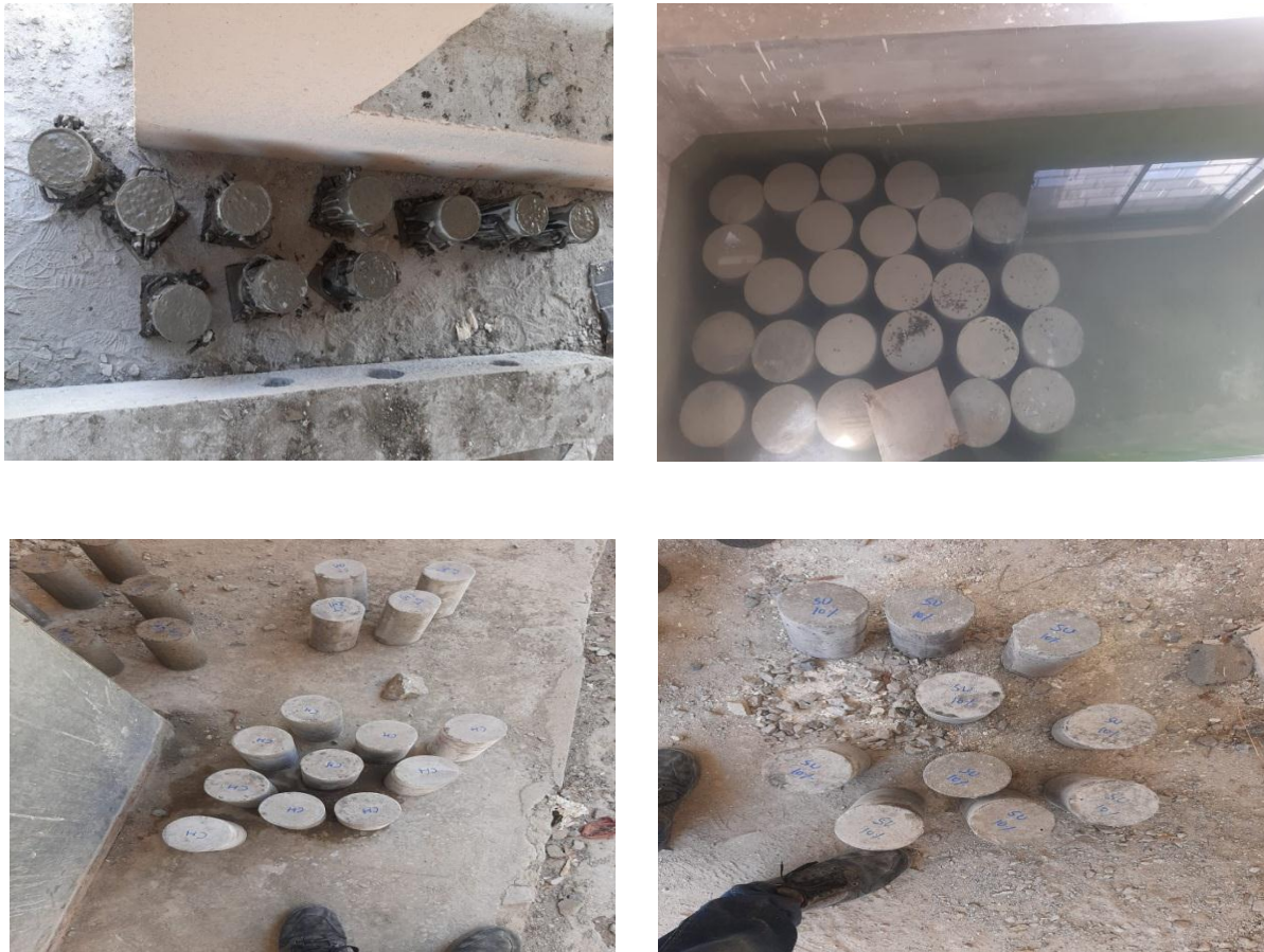
Figure 3.6 Preparation of specimens and curing
