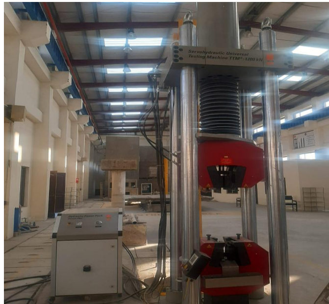
Figure 3.11 Compression testing machine
