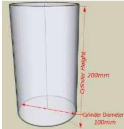
Figure 3.9 Cylinder size and dimensions
