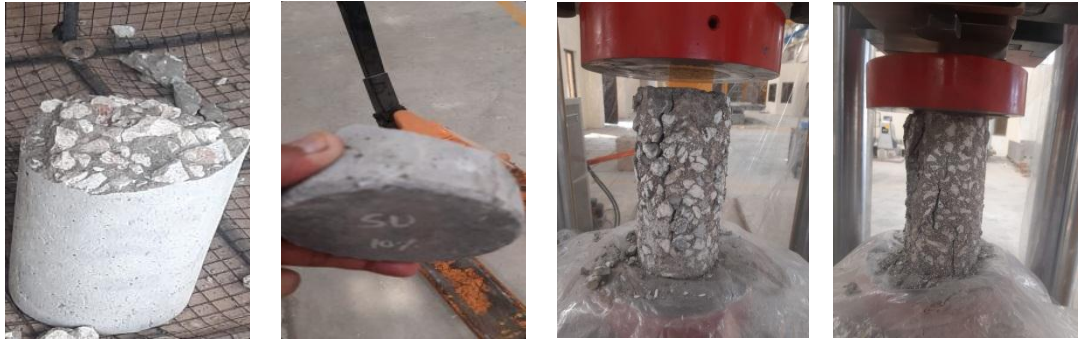
Figure 4.5 Failure modes of concrete samples on all temperatures
