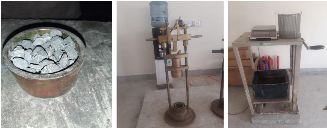
Figure 3.4 Test setups for physical properties of aggregates
