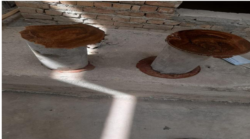
Figure 3.7 Capping of specimens
