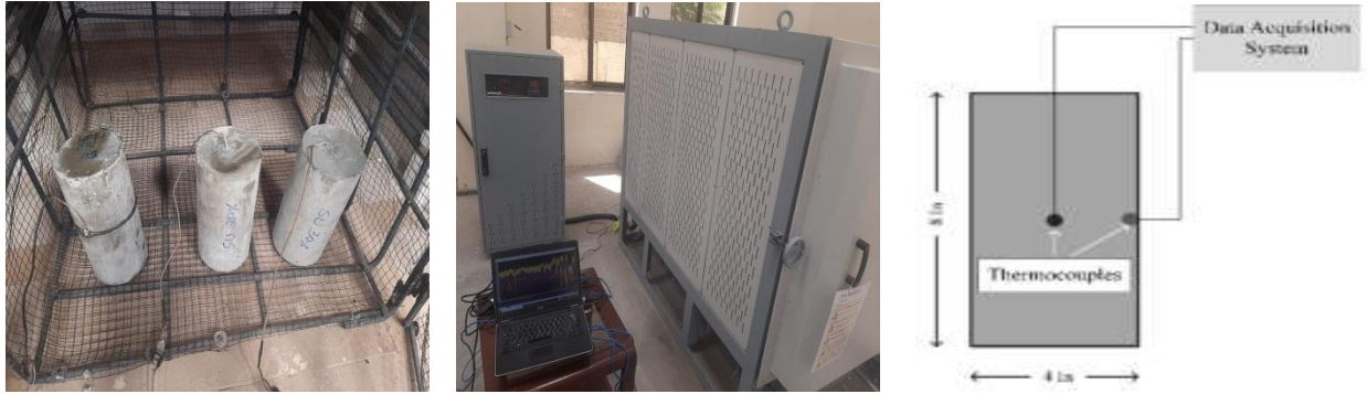
Figure 3.8 Instrumentation process and a schematic diagram to demonstrate the heating characteristics
