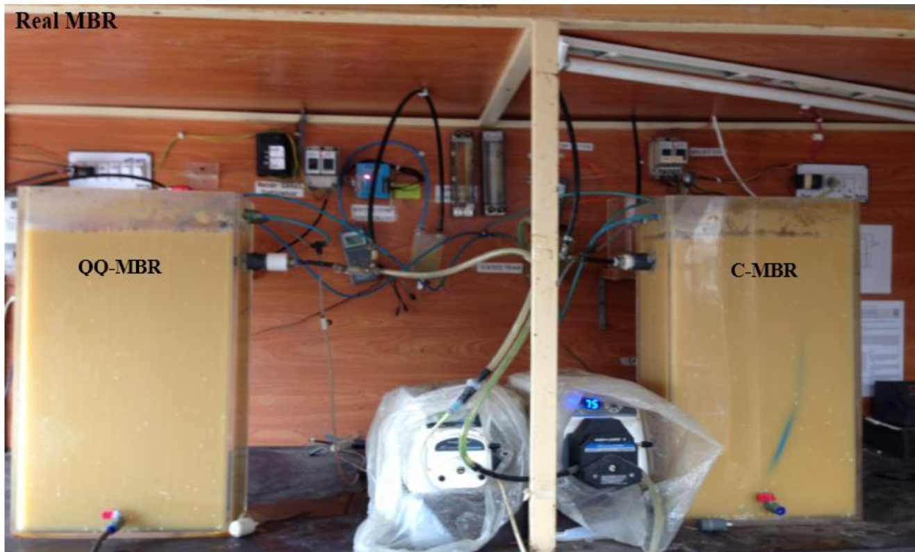
Figure 3.3 Semi pilot-Scale MBR at NUST water and wastewater lab
