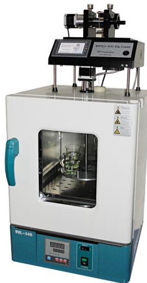
Figure 3-2 Dip Coater (WPTL6-0.01 by MTI).
