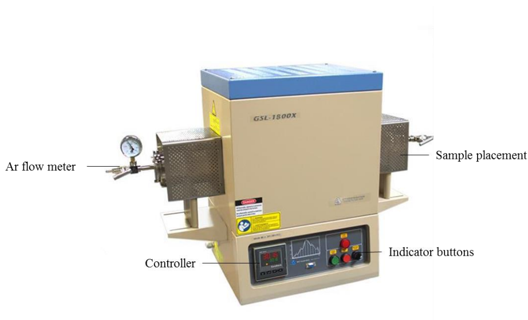
Figure 4-6 MTI GSL 1600 tube furnace.
