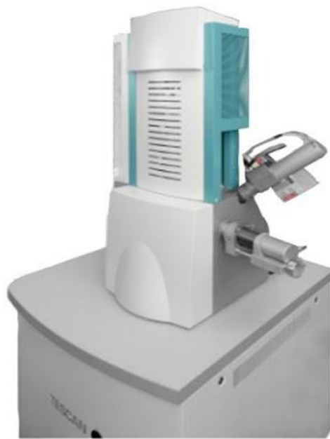
Figure 3-3 TECASN Vega 3 Scanning electron microscopy.
