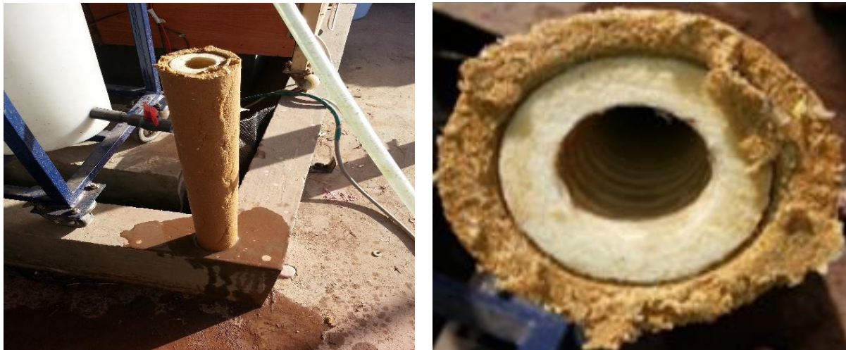
Figure 3.6: Cartridge filter after clogging
