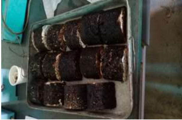
Figure 3. 22: Schematic of SCB test
