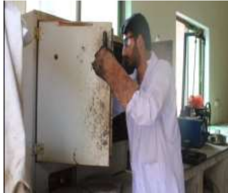
Figure 3. 14: Pre-Heating of Aggregate and Bitumen
