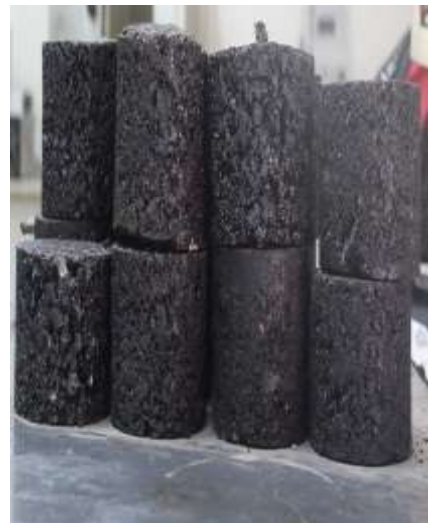
Figure 3. 17: Marshal Sample Preparation
