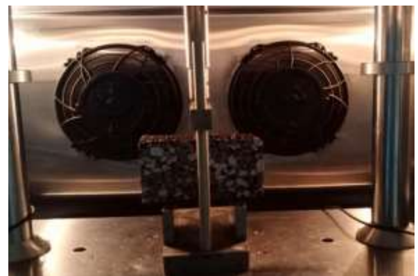
Figure 3. 23: Schematic of 3 point bending test
