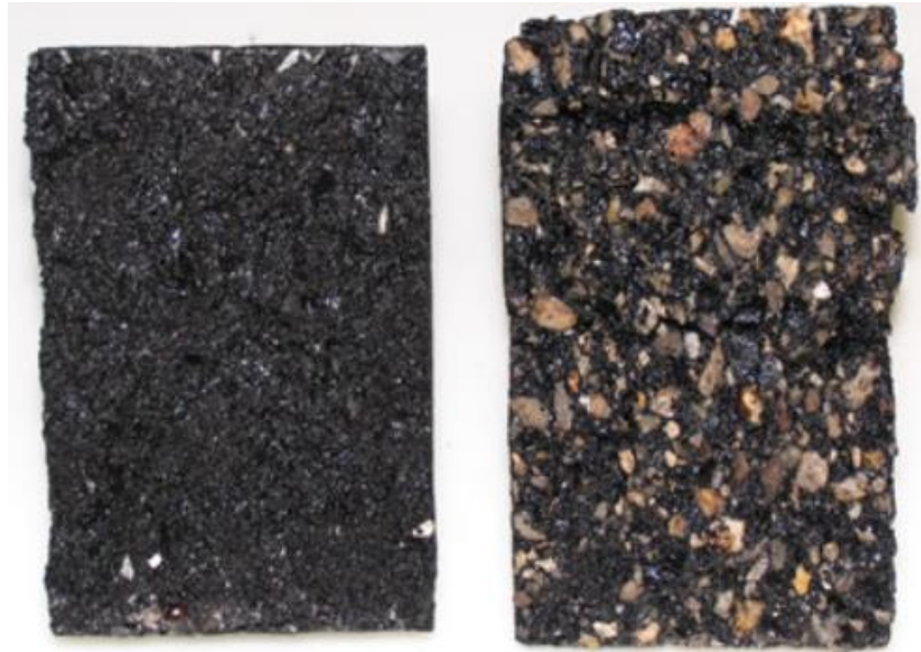
Figure 2.2: HMA samples with no moisture damage (left) and moisture damage (right) (Hicks, R.G. (1991))
