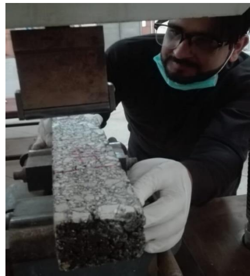
Figure 2.3: point Bending Beam Test performed in UTM
