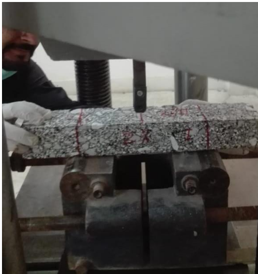
Figure 2.3: point Bending Beam Test performed in UTM
