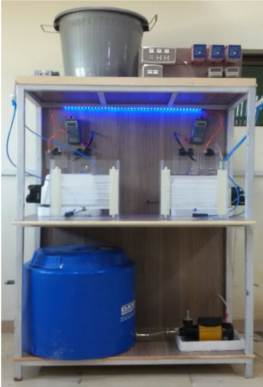
Figure 3.2: Lab Scale MBR without sludge
