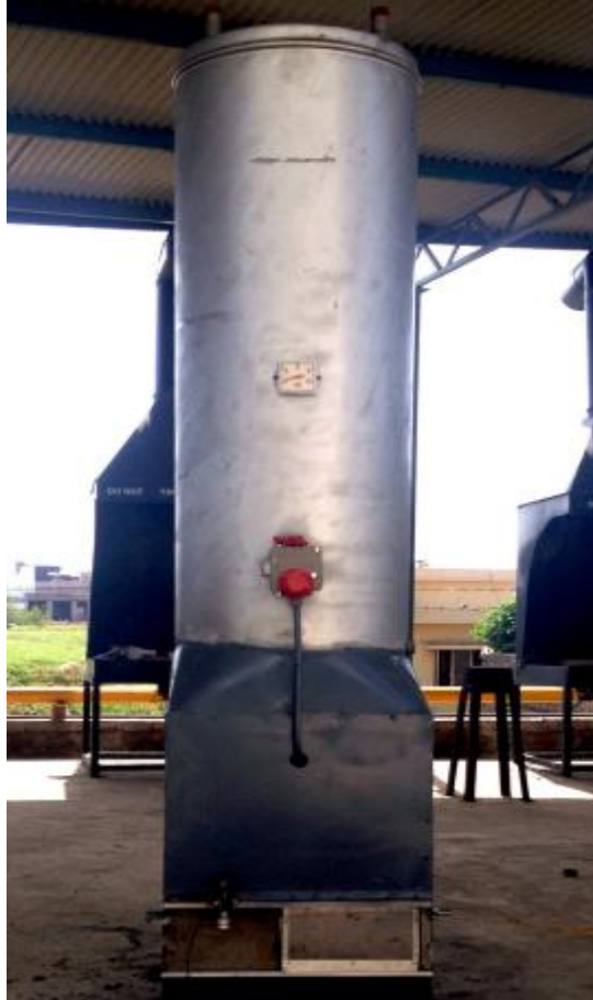
Figure 4.8: Furnace final Design: involving fuel combustion chambers and hot water storage tank coupled
