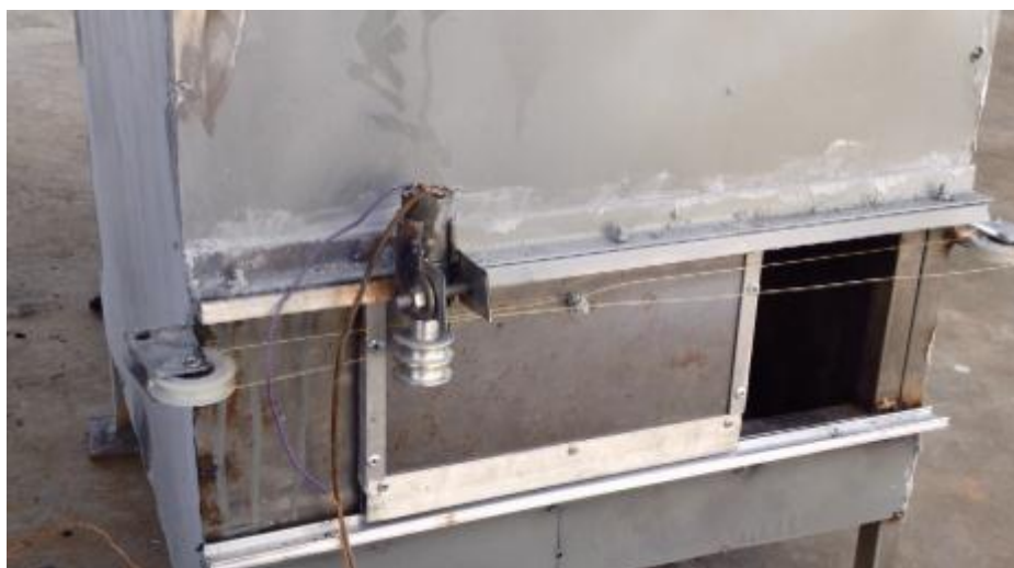
Figure 4.9: Air ventilation sliding mechanism
