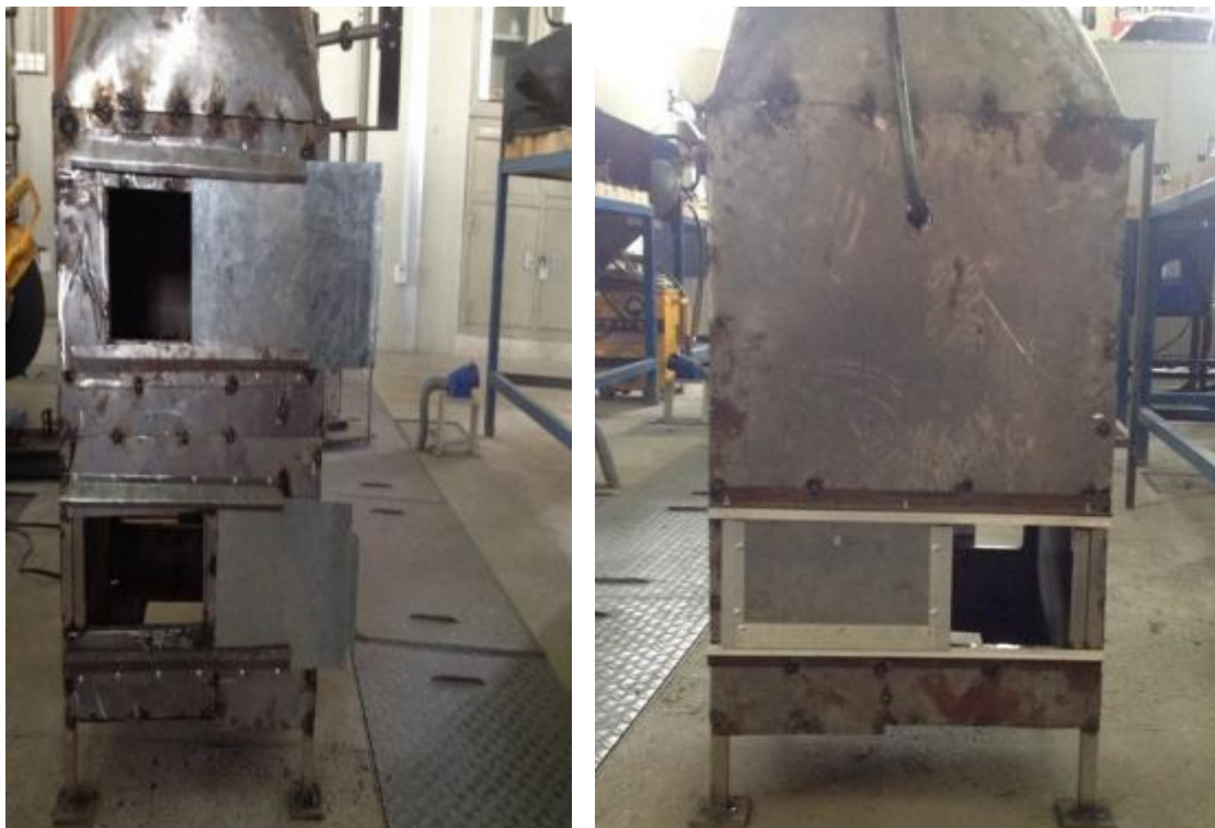
(a) Fuel charging door (upper) and furnace cleaning door (lower)
