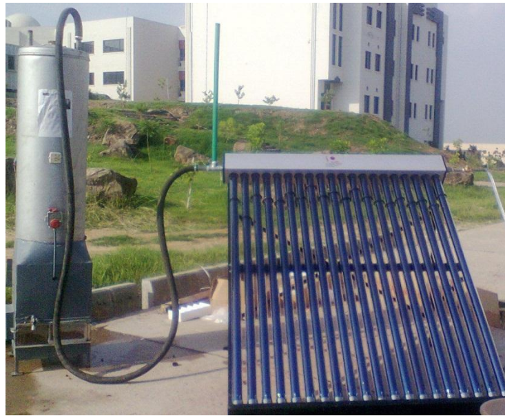
Figure 4.4: Heat pipe evacuated tube solar thermal manipulate connected with multi-fuel furnace
