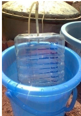
Figure 3.4: Water displacement setup for measuring volume of biogas
