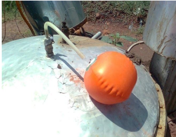
Figure 4.7: Football bladder filled with biogas
