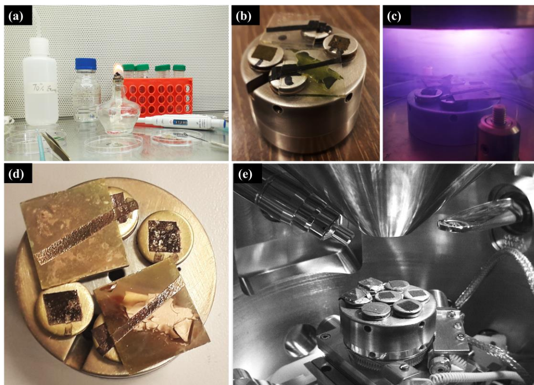
Figure 3.6 Microalgal step-by-step sample preparation for SEM examination.
