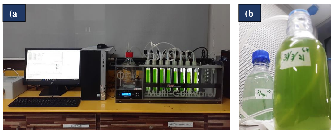
Figure 3.3 Algal cultivation in Multi-Cultivator (a) and PBR (b) for Growth kinetics study.
