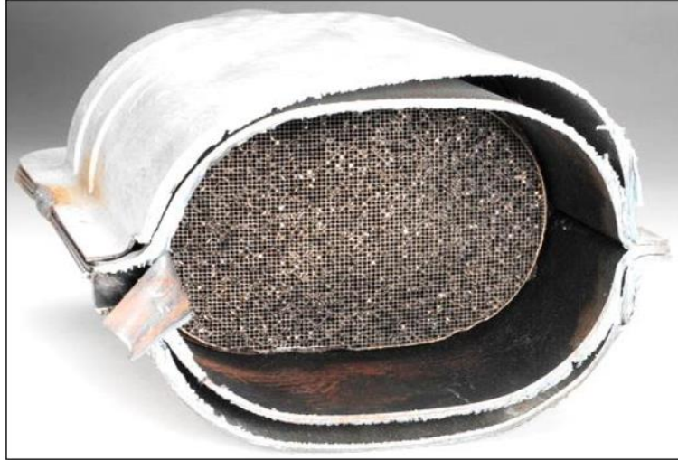
Figure 2: Fouling of a CC (Eastern Catalytic, 2013)
