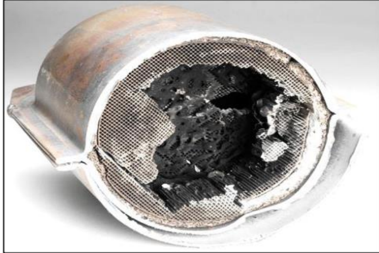
Figure 3: A Corroded CC (Eastern Catalytic, 2013)
