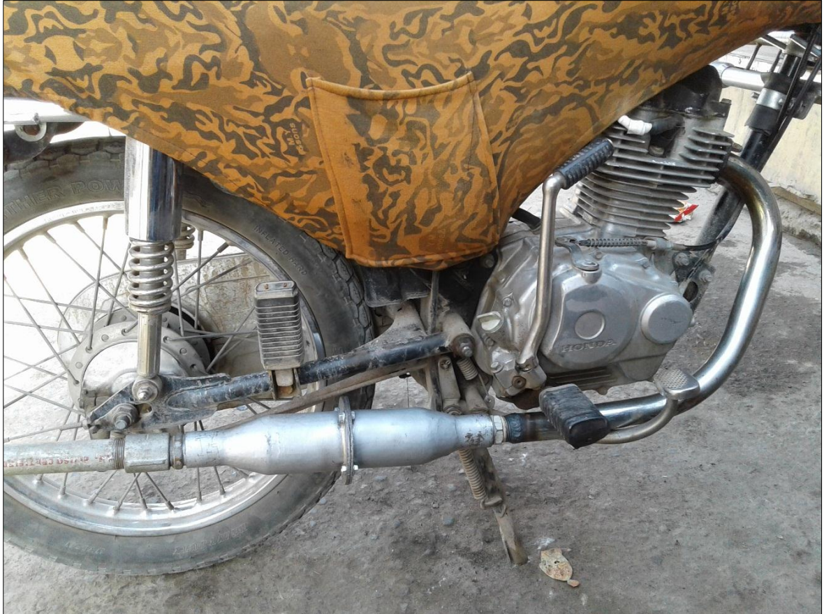
Figure 3.6. Catalytic converter installed at 125 cc Motorcycle
