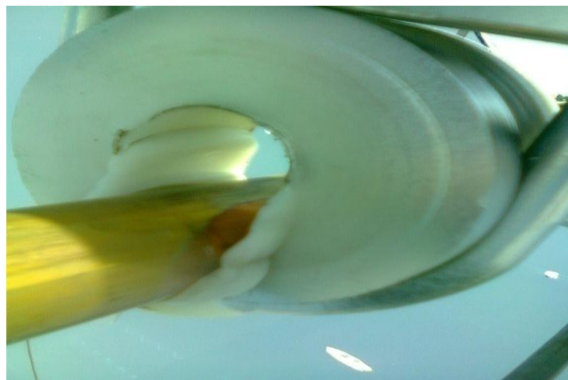
Fig. 4. 12 The melted Teflon ring due to very high temperature
