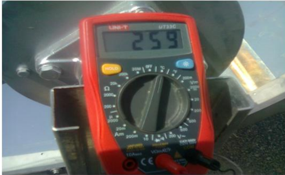
Fig. 4. 13 The temperature at instant when Teflon got melt
