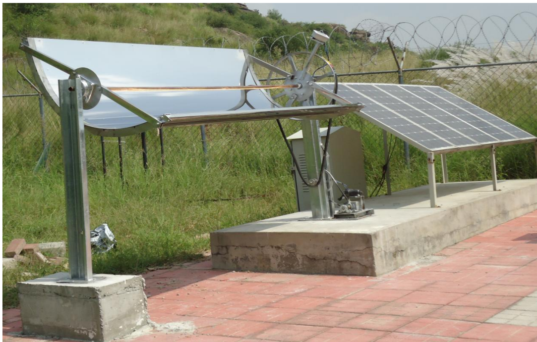
Fig. 4. 11 The receiver tube of parabolic trough at its full focus
