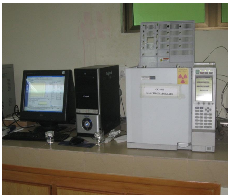
Figure 3.1: Shimadzu 2010 Gas Chromatogram coupled with ECD
