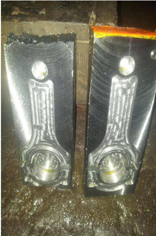
Figure 3-11 Connecting Rod manufacturing
