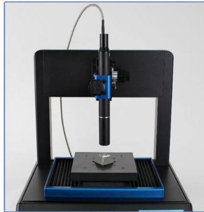
Figure 3-13 A non-contact profilometer
