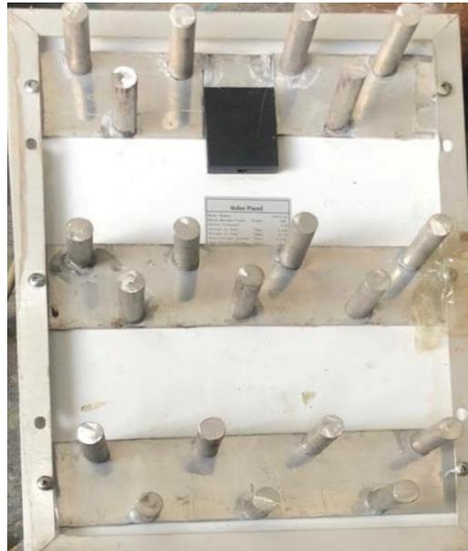
*Figure 4-1 Circular fins attached on the back of the PV module*
