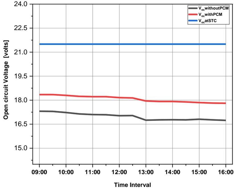
Figure 6-2 Electrical improvement of open-circuit voltage
