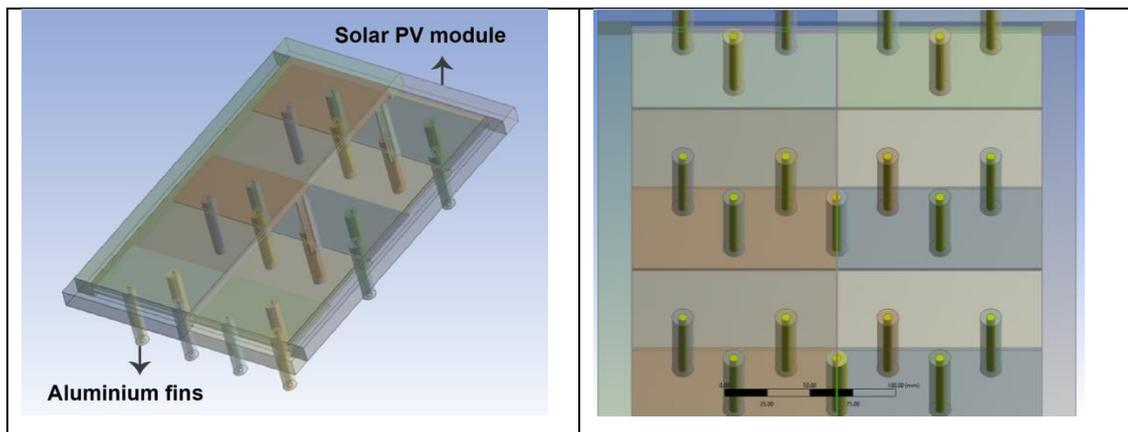
Figure 5-1 3D model Solar Panel with attached fins
