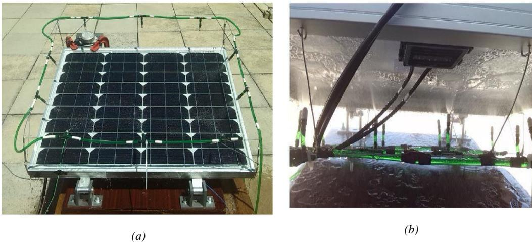
Figure 2-6 Water spray cooling method [24]
