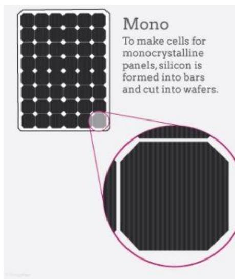
Figure 2-1 Monocrystalline PV module[14]
