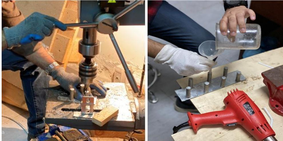
*Figure 4-2 Drilling of fins and encapsulation with PCM*
