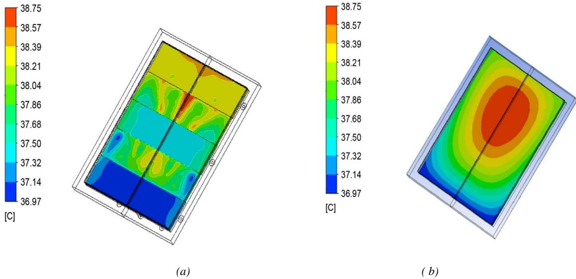
Figure 6-4 Comparison of tedlar wall temperature between fin and unfinned PV module
