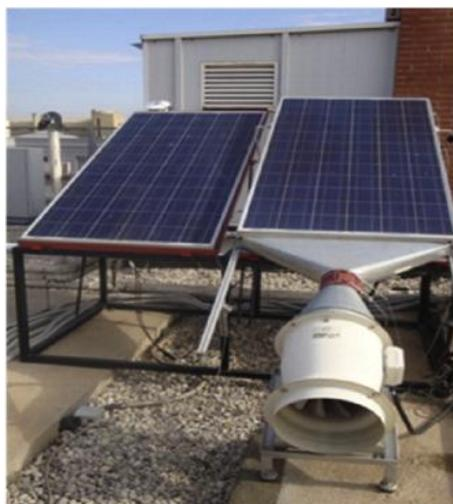
*Figure 2-5 Advanced air-based cooling technique [23]*
