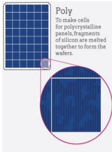
Figure 2-2 Polycrystalline PV module [14]
