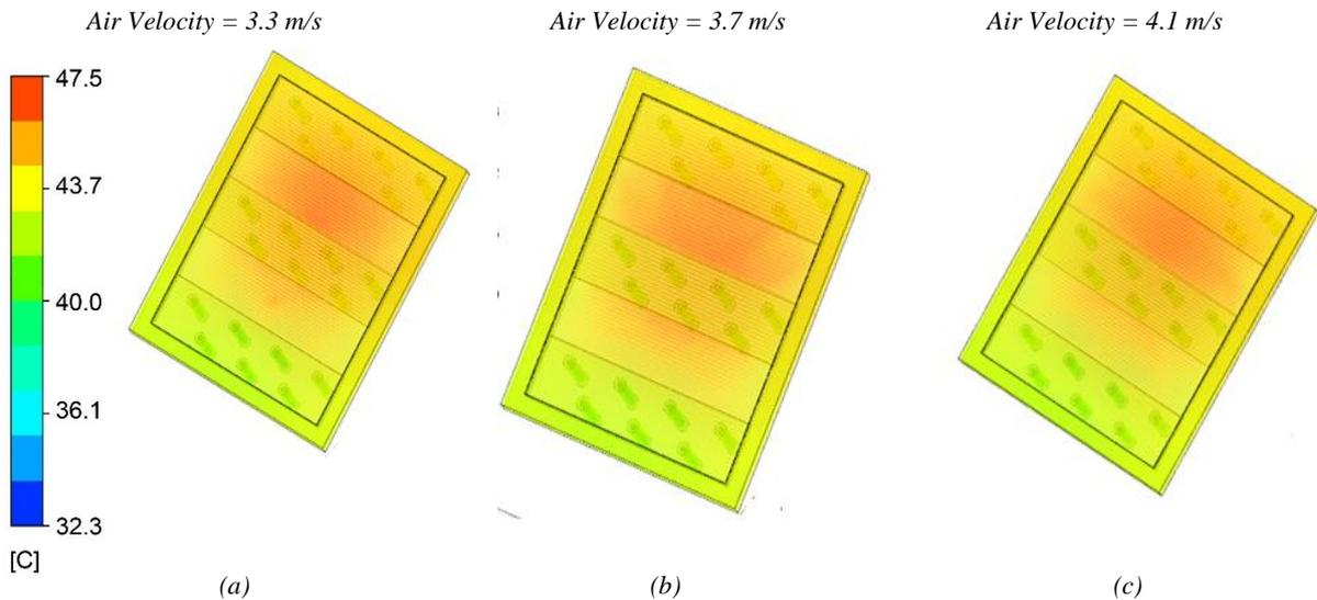
Figure 6-6 Different velocities distribution profiles on solar PV module
