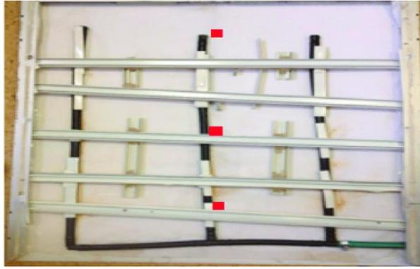
*Figure 2-7 Backside water cooling system[26]*
