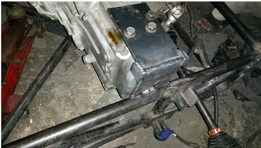
Figure 4.6 Left engine mounting
