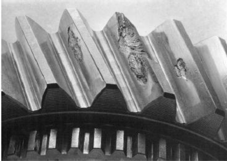
Figure 2.6 Macropitting due to flank surface fatigue
