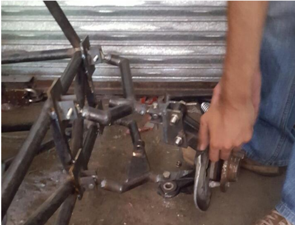
Figure 4.3 Modified hub and wishbone assembly
