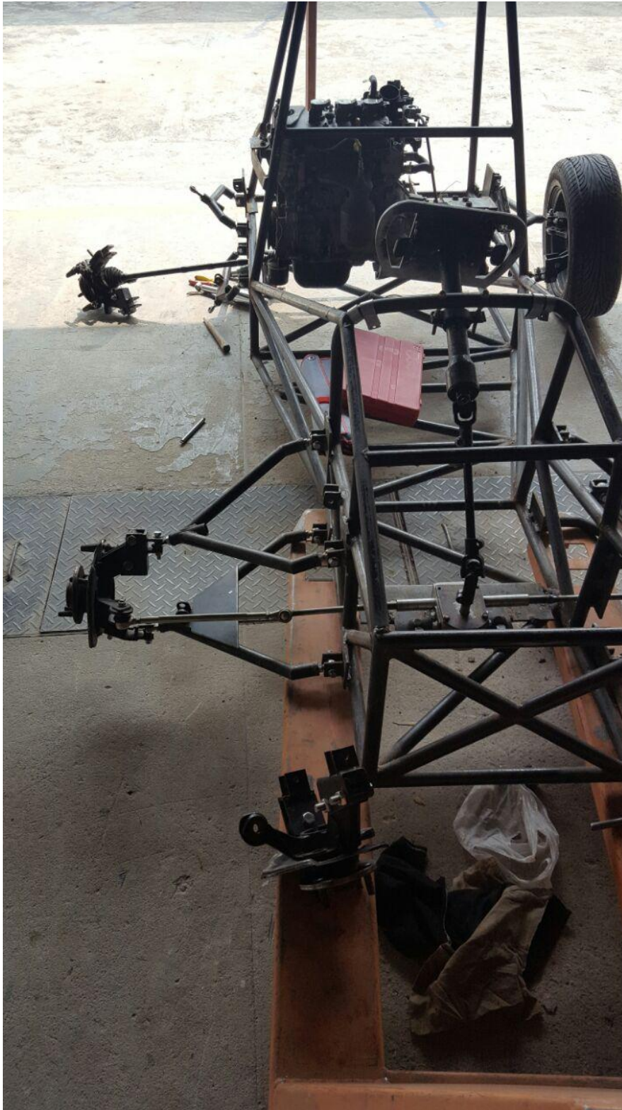
Figure 4.9 Mounting the suspension and tires onto the frame
