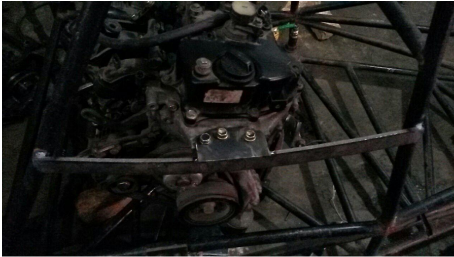
Figure 4.7 Right engine mounting
