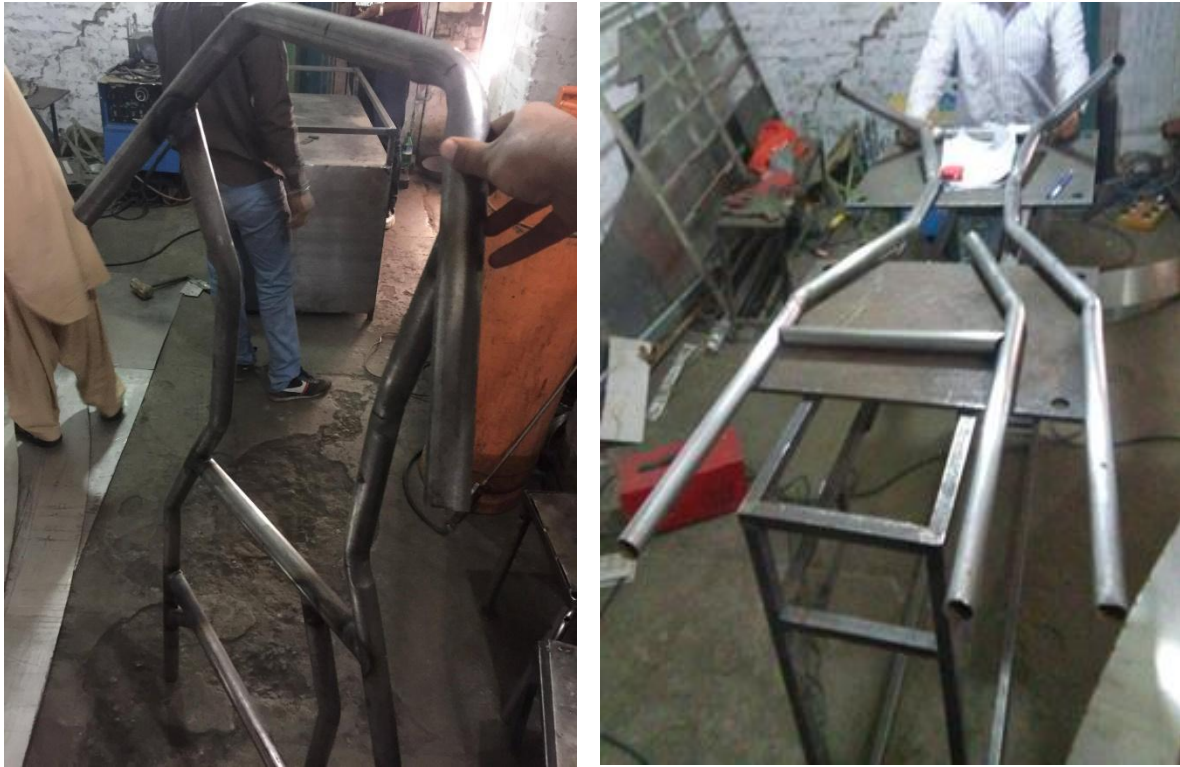
Figure 5.1 & Figure 5.2 Representing the making of Chassis in the welding shop
