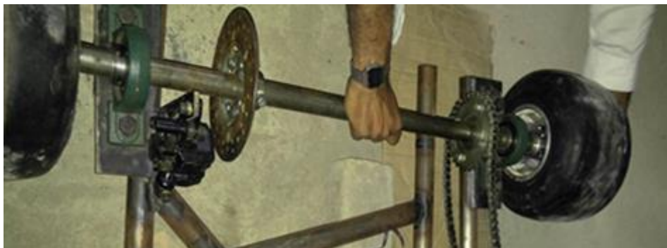
Figure 5.9 Rear Shaft with Journal Bearings mounted as well as Sprocket & Brake Disc
