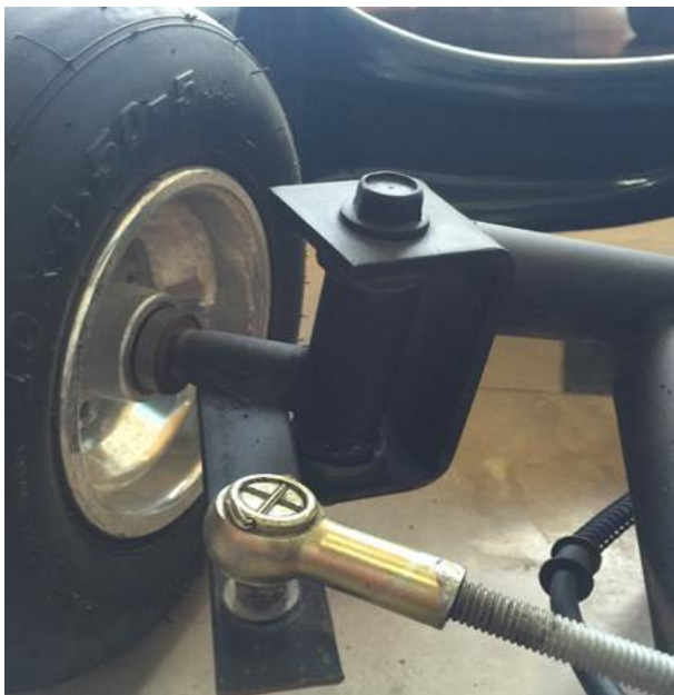
Figure 5.5 & 5.6 clearly show that there is no suspension used in the Go-Kart
