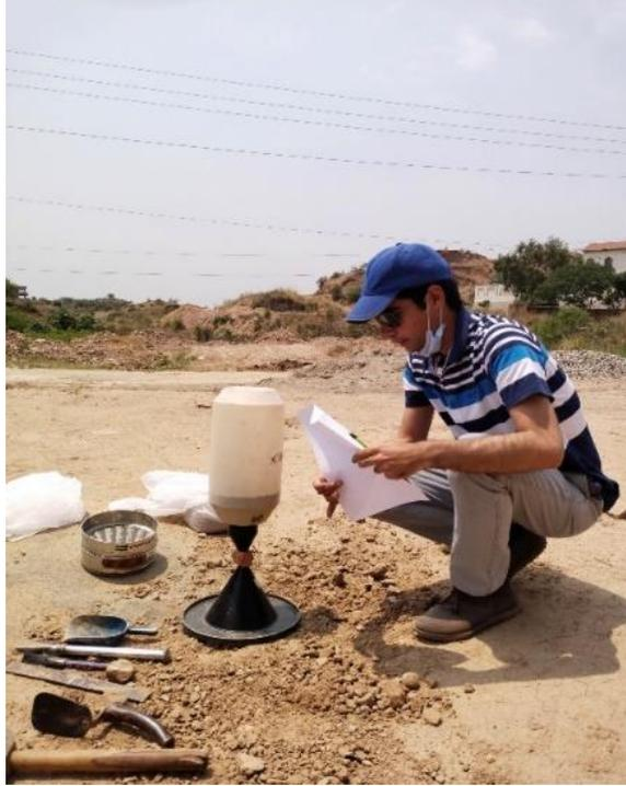
Figure 3.8 In situ soil density measurement
