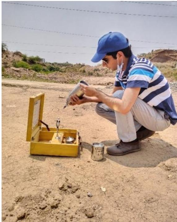
Figure 3.9 In situ moisture content measurement
