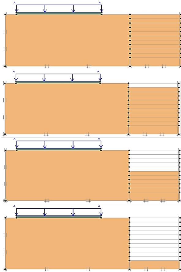
Figure 3.16 Staged Excavation at 1 m intervals
