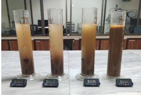
Figure 3.13 Hydrometer test
