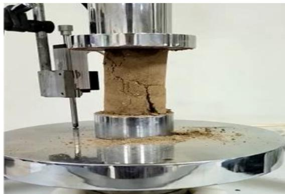
Figure 3.14 Unconfined Compression Test
