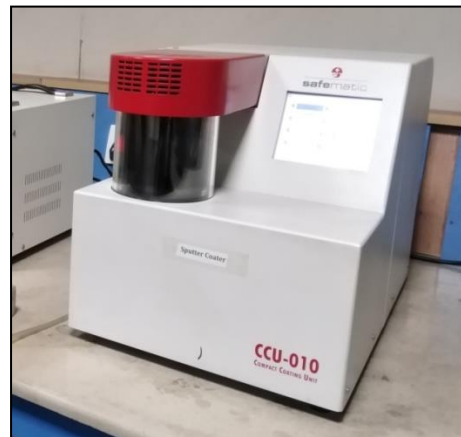
Figure 3-21: Compact Coating Unit
