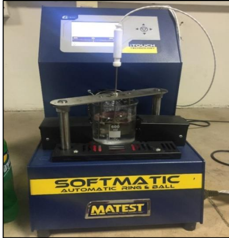
Figure 3-12: Ring and Ball Apparatus Figure 3-13: Samples for Softening Point
