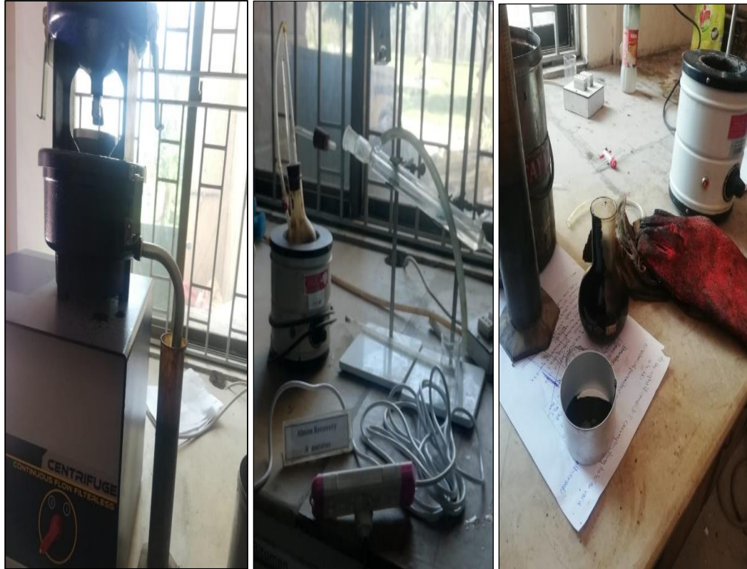
Figure3.5: Extraction and Recovery of RAP binder using Abson method
