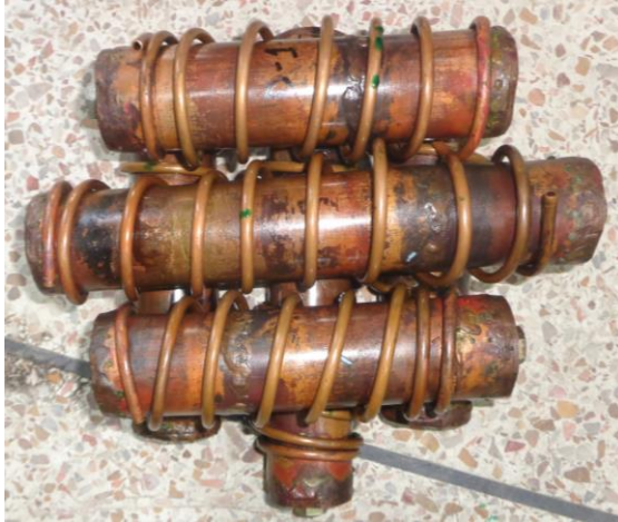
Fig. 3.4. Encapsulated PCM arrangement in rows
