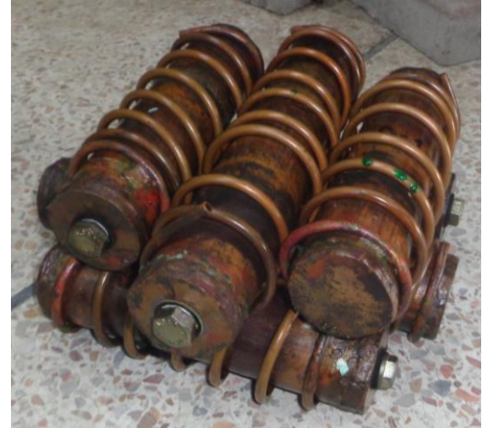
Fig. 3.4. Encapsulated PCM arrangement in rows
