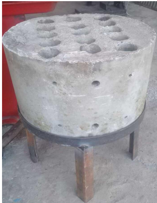
Fig. 3.5. Concrete block with radial and axial holes
