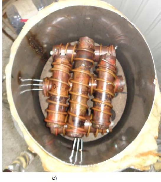
Fig. 3.7. Storage tank with thermocouples in radial and axial direction a) outer view b) and c) inner view of TES unit
