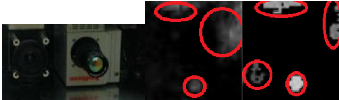
Figure 8: An off the shelf IR camera with PCI Board, A typical image after resampling and final output.
