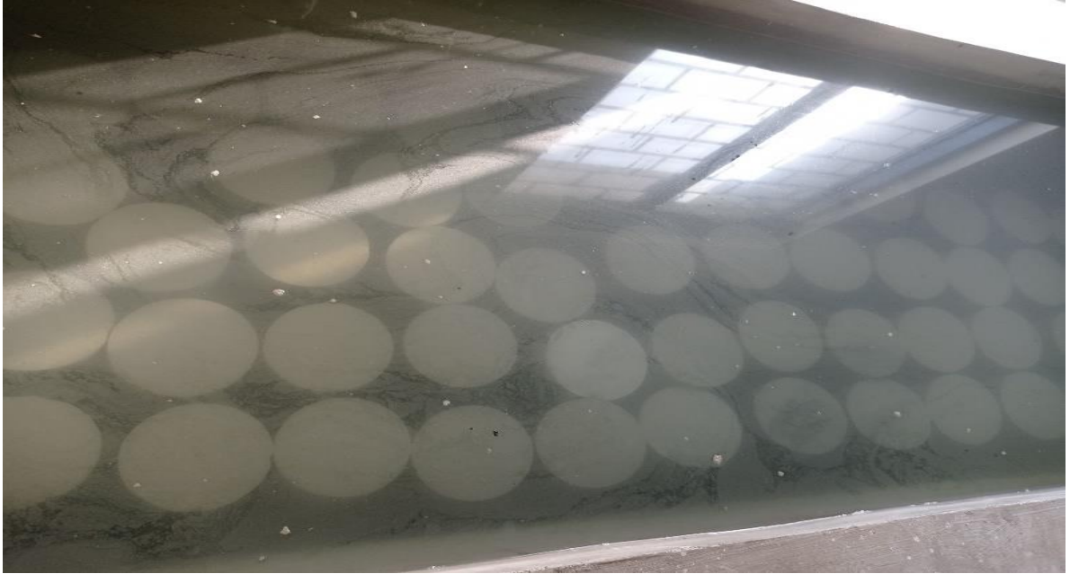
Figure 7A: Curing Phase of Cylinders
