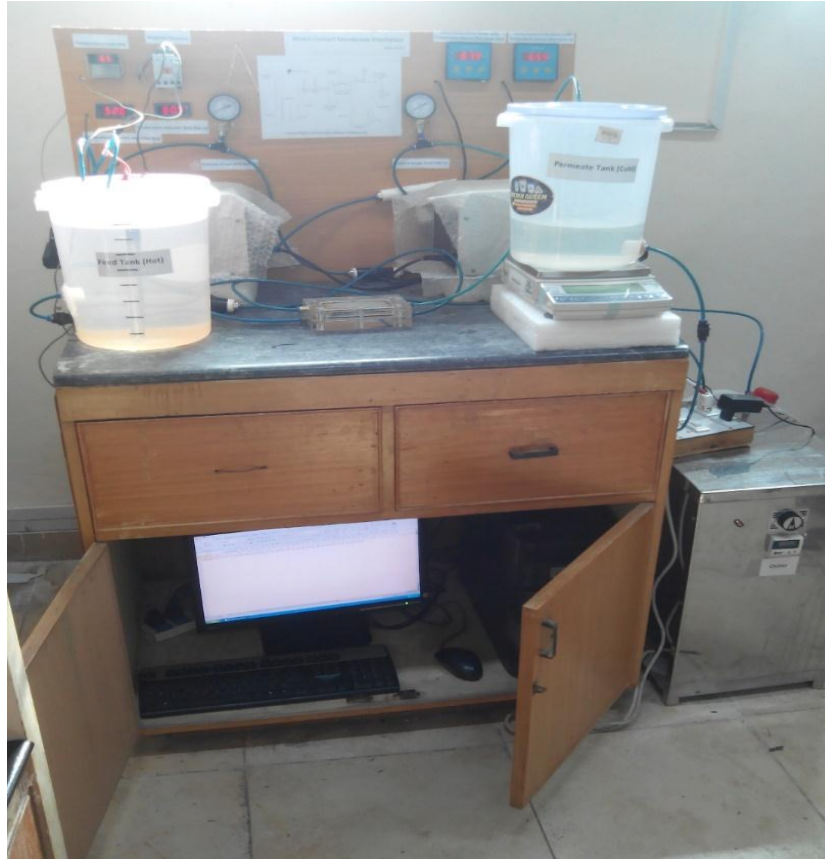
Fig. 16. Lab scale direct contact membrane distillation system at IESE, NUST
