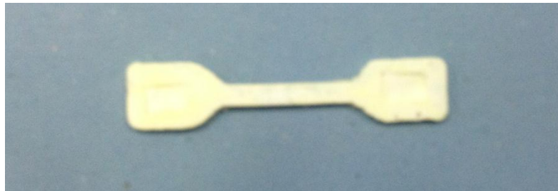
Figure 4.7 Photograph of dumb bell shaped specimen for flexural property test
