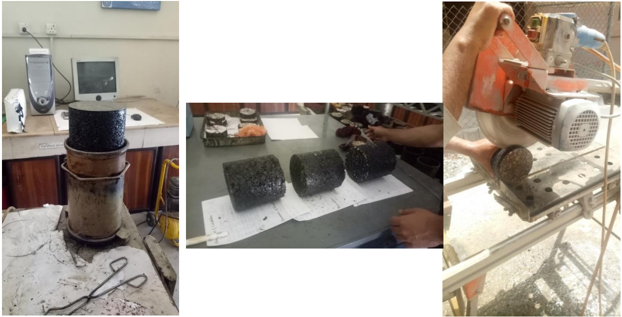
Figure 3.18 Gyratory sample preparation & Saw Cutting
