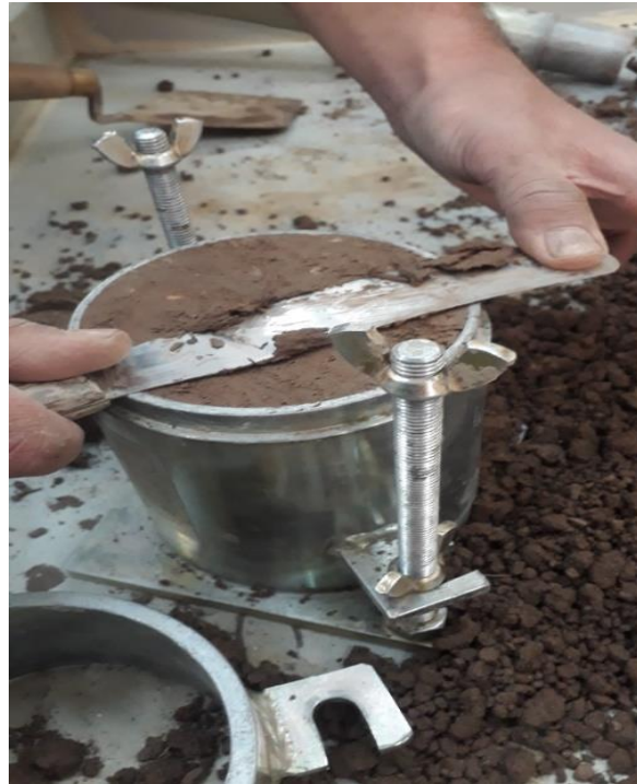
Figure 2. Trimming compacted soil in the standard proctor mold
