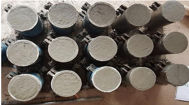
Figure 20 Samples for Compressive Strength
