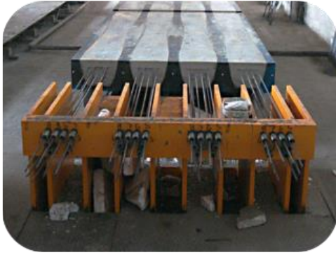
a) Prestressed Concrete
