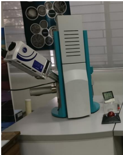
Figure 3.7 Image of SEM and schematic diagram of its working mechanism.[12]
