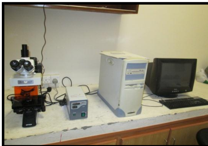
Figure 3.10: Fluorescent Microscope for Visual Analysis
