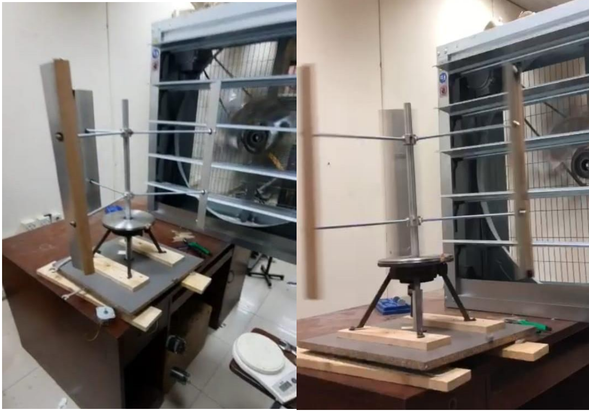
Figure 32: torque (left) and RPM (right) testing
