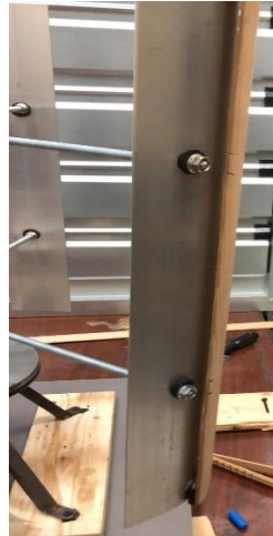
Figure 23: Slats integrated with turbine blade
