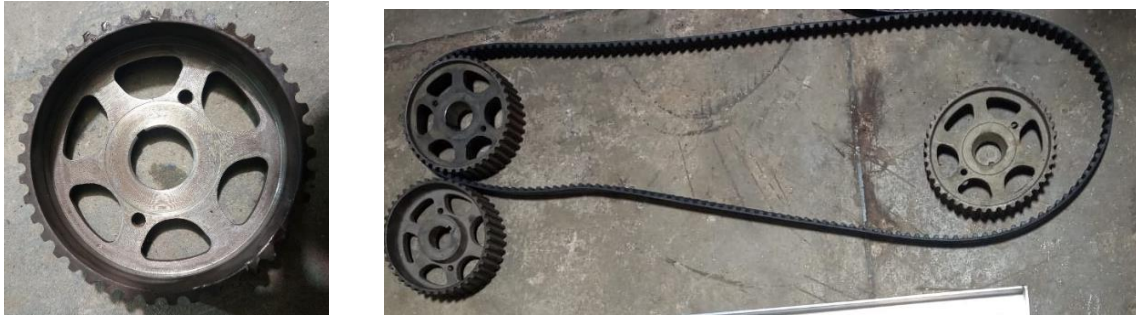
Figure 22: Tire machined out of Car gears, and its tracks
