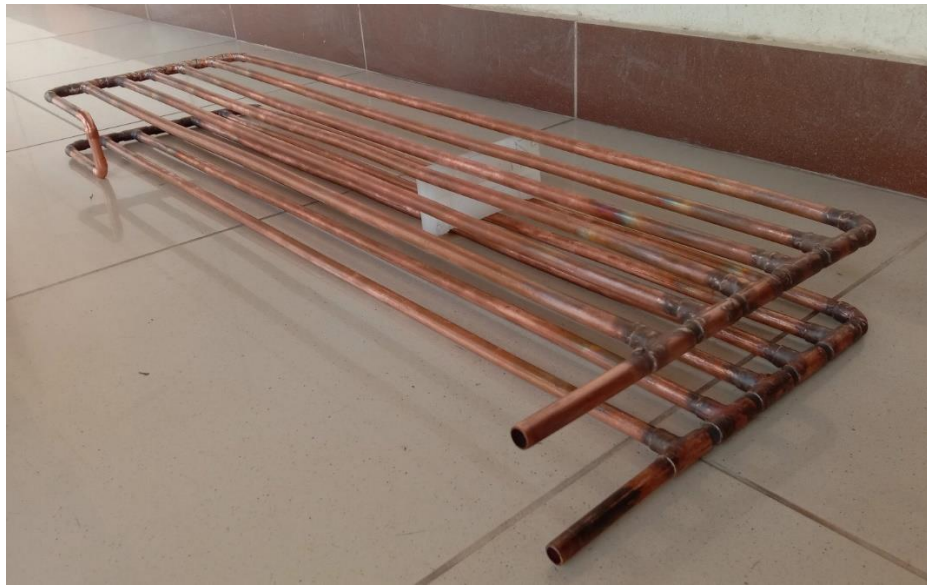
Figure 3. 8 Absorber heat exchanger
