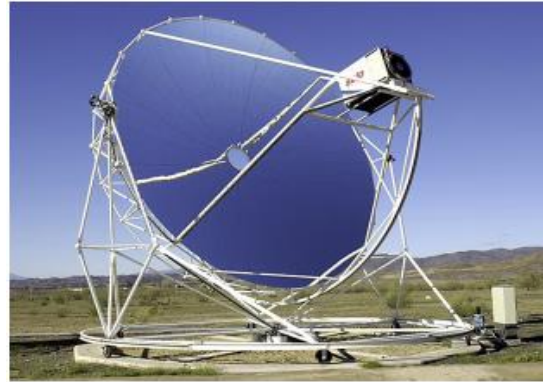
Figure 2. 10 Parabolic dish reflector
